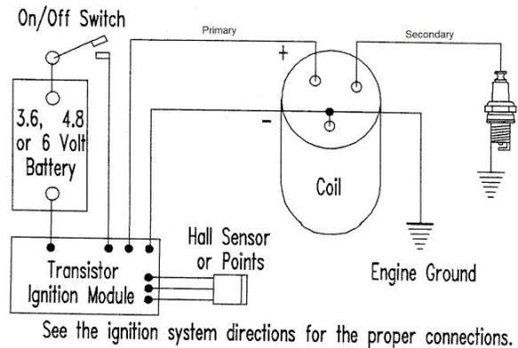
Example Using a TIM-6 Transistor Ignition Module
